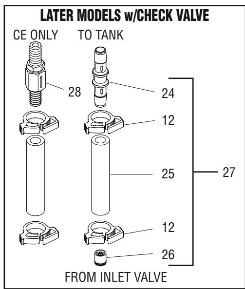
**NOTE:** LETTERING ON FLOW WASHER MUST FACE TOWARDS THE INLET
